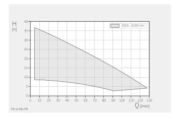
Specifications apply for water at 20°C Within the characteristic diagrams, each operating point is possible through parametrisation of the drive.
