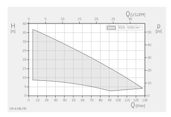
Specifications apply for water at 68°F Within the characteristic diagrams, each operating point is possible through corresponding parametrisation of the drive.
