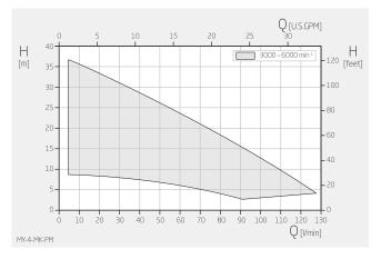
Specifications apply for water at 68°F Within the characteristic diagrams, each operating point is possible through corresponding parametrisation of the drive.
